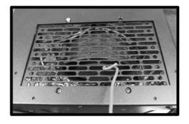
Use a wire to hook the perforated vent plate
